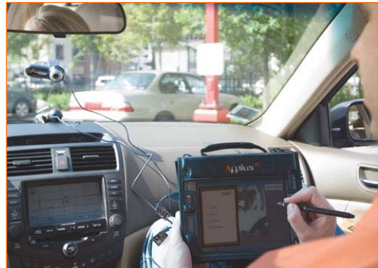
The Applus+ DrivewAtch™ unit in use. Dual cameras attach to the windshield to record video of the driver's view as well as the vehicle's interior.
