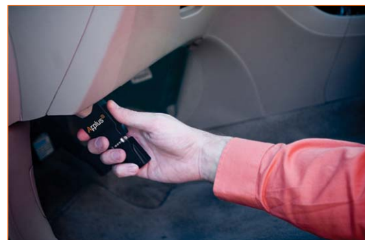
A wireless OBD connection transmits data from the vehicle to the DrivewAtch™ portable Tablet PC.
